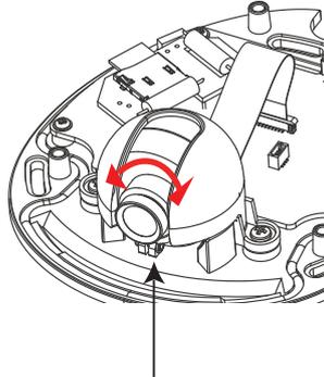
Tighten the lens lock screw.
