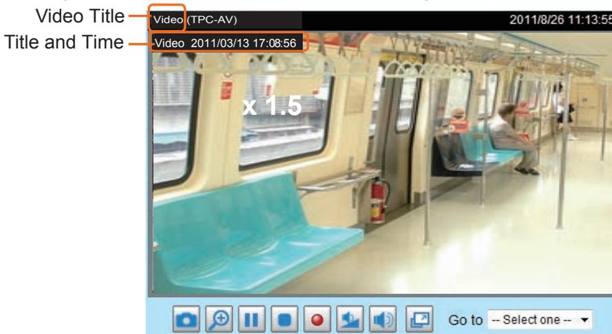
**Video orientation:** Flip--vertically reflect the display of the live video; Mirror--horizontally reflect the display of the live video. Select both options if the Network Camera is installed upside-down (ex. on the ceiling) to correct the image orientation. Please note that the preset locations will be cleared after flip/mirror.
