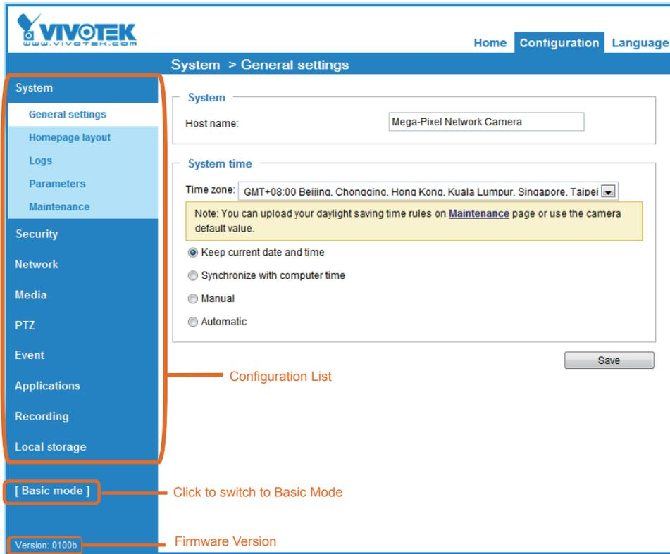
Each function on the configuration list will be explained in the following sections. Those functions that are displayed only in Advanced Mode are marked with **Advanced Mode**. If you want to set up advanced functions, please click on **Advanced Mode** at the bottom of the configuration panel to quickly switch over.
