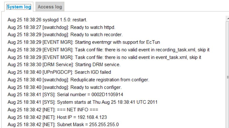
This column displays the system log in chronological order. The system log is stored in the Network Camera's buffer area and will be overwritten when reaching a certain limit.
